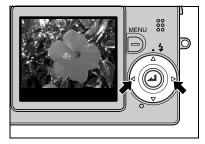
3 Press the ♠ side of the zoom button to enlarge the image and the ♣ side to return the enlarged image to its original size.
